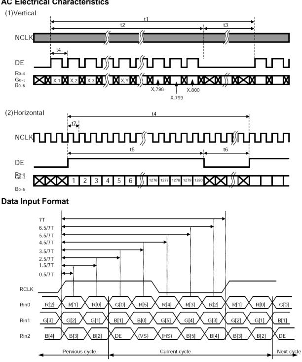
LVDS Receiver Input Timing Definition for 6bits LVDS input
