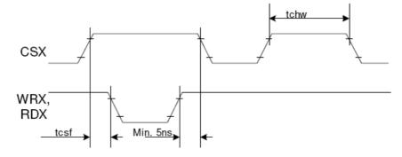
Note: Logic high and low levels are specified as 30% and 70% of VDDI for Input signals.
