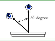
Under daylight lamp 20  $\sim$  40W ,  $\,$  product distance inspector 'eye 30cm,incline degree 30°  $_{\circ}$
