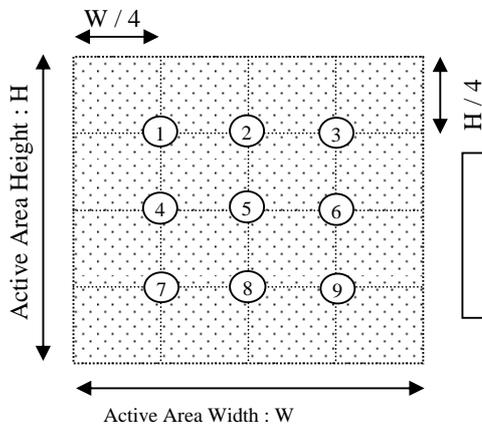
$$\text{Brightness Uniformity} = \frac{\text{Minimum Brightness of Point 1~9}}{\text{Maximum Brightness of Point 1~9}}$$
