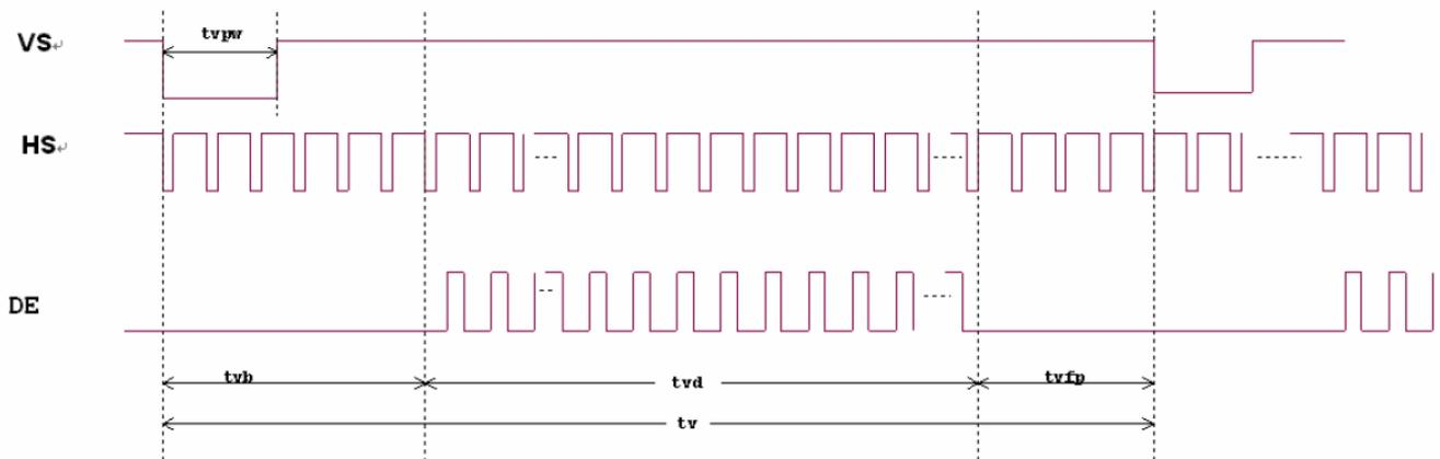
Vertical input timing diagram
