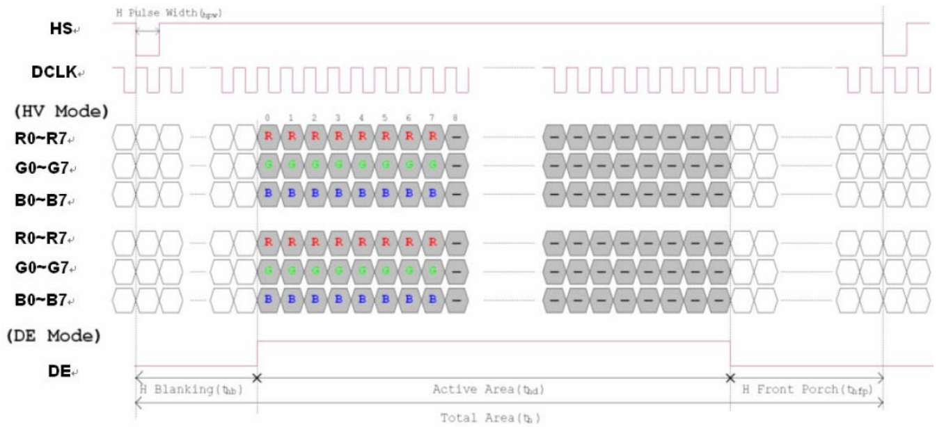
Horizontal input timing diagram
